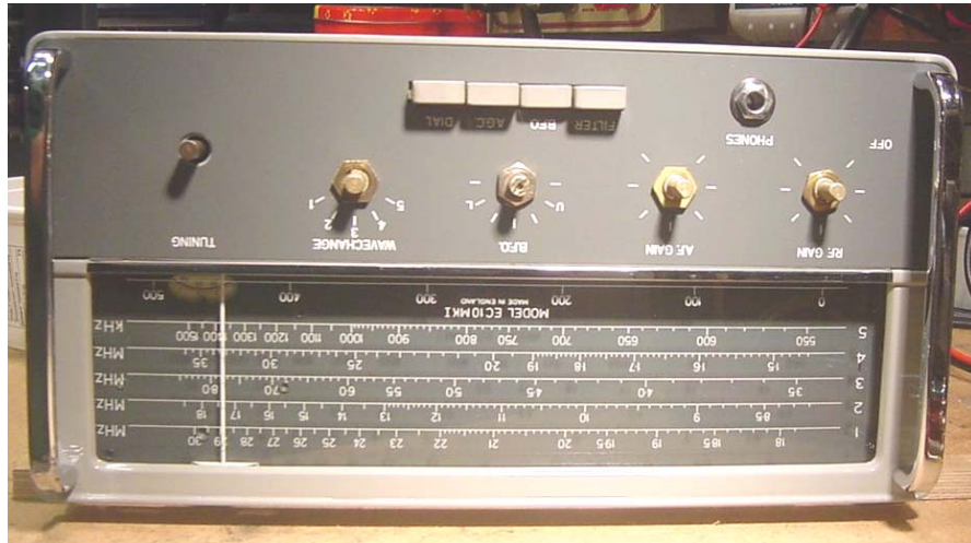
Above: Fitting the new fingerplate – take care when tightening those shaft nuts!
